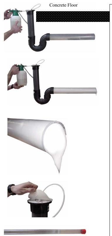
Floor drain tests have been completed to record time and volume. The picture shows a standard drain complete with trap. This is a 4-inch diameter pipe with an overall length of 62 inches. From the top of the drain pipe inlet to bottom of the trap is 19 inches.
